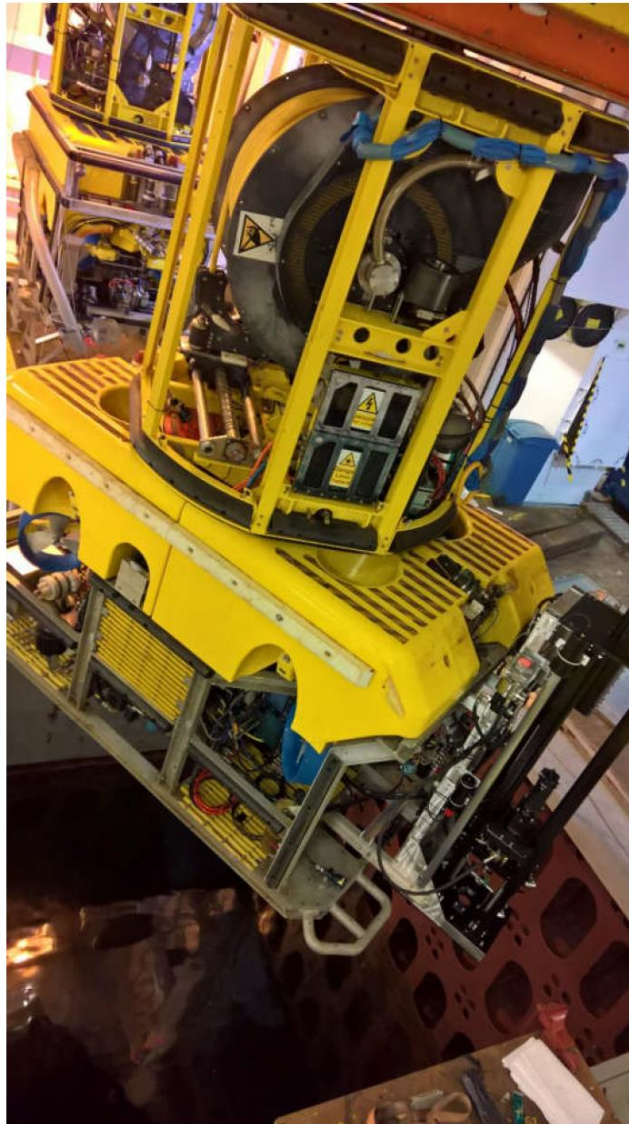
Figur 1 ROV with drill rig during moonpool launch prior to testing
