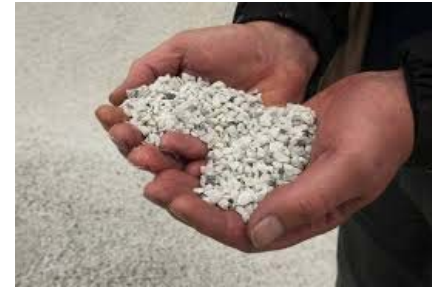
Anorthosite is a feldspar rock consisting almost entirely of alumina (30%), calcium oxide (15%) and silicon oxide (50%)
