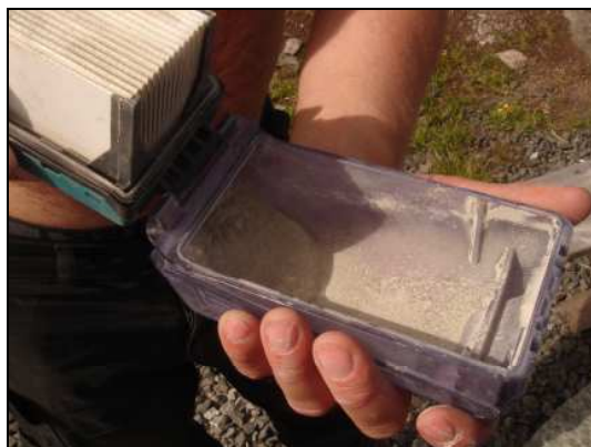
Figure 10-22. Dust Sample After Drilling
