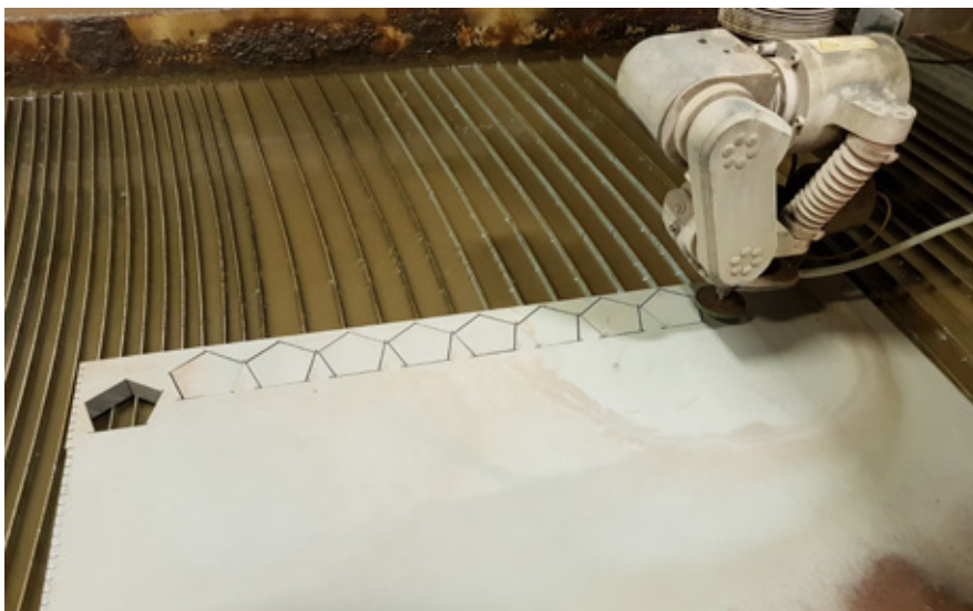
Garnet is the main abrasive mineral used in waterjet cutting.
