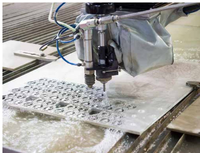
Garnet is the main abrasive mineral used in waterjet cutting.
