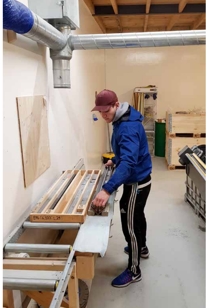
Drill core inspection and logging at the Engebø combined office and project coordination facilities.
