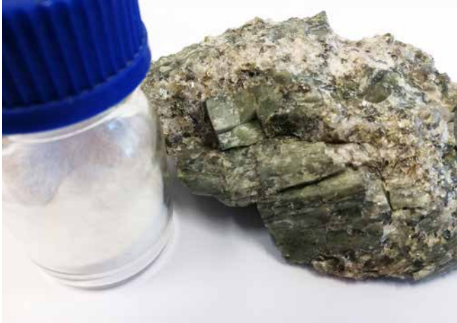
Lithium carbonate test sample originated from spodumen pegmatite.
