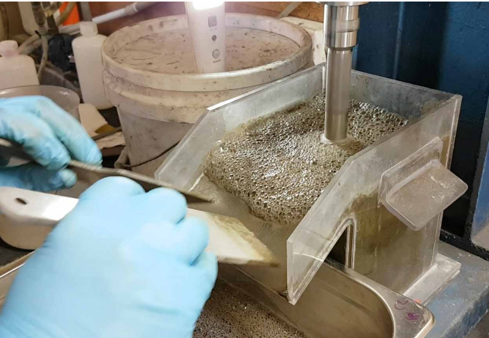
Flotation test work for optimisation of rutile recovery at Core Resources, Australia.
