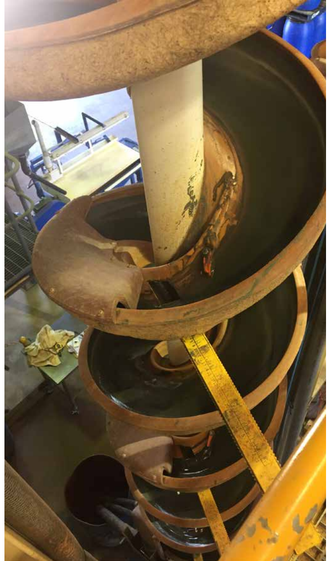
Gravimetric separation test work at IHC Robbins, Australia.
