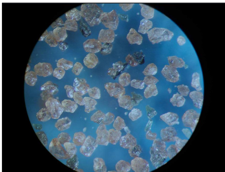
Figure 11-19: Microscope Image of the Coarse Garnet Product from Programme 1308
